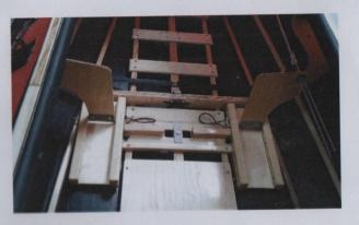
• Put the footplate aft the n°3 crossrib (red marks) for solo trim.
