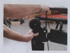
• The rudder leverage black cord has to be stretched along the starboard side. Connect it to the plastic hook with elastic (inset). The elastic will keep the cord in tension.
