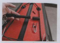
• The rudder bar has a moveable ring. Get it out by unscrewing the shackle.
