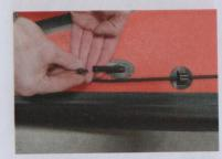
• Get the rudder line exit tube tops off.
