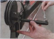
• Get the bar into the rudder hole on starboard.
