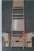
Put the pedal plate against the first wood plate
